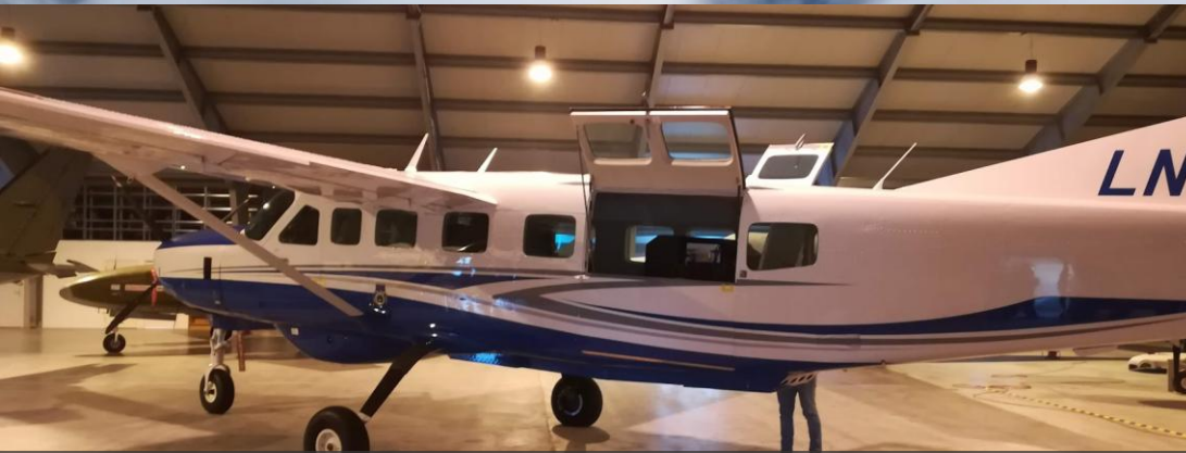
2x Cessna 208b Grand Caravan aircraft with 2 hatches. ALB Speed: 120-140 knots (220-260km/h). ALB Flying Height: 400-600m.
