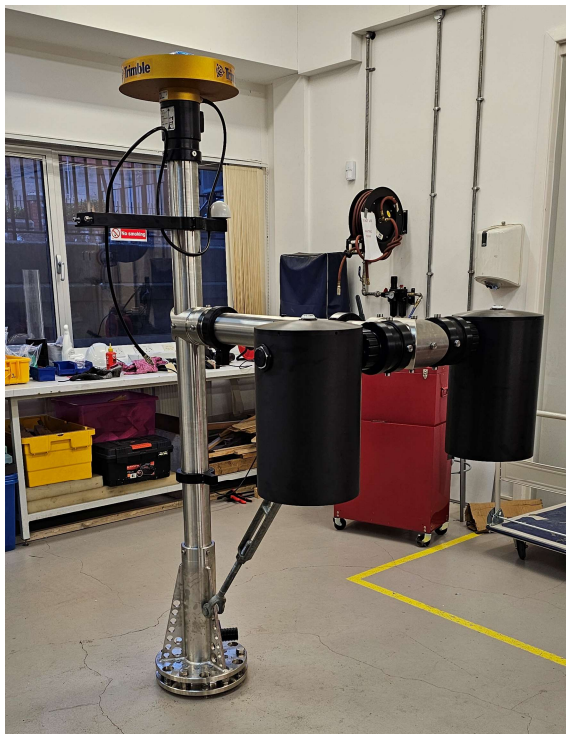
NOC GNSS & Radar Tide Gauges designed and built in NOC Liverpool
