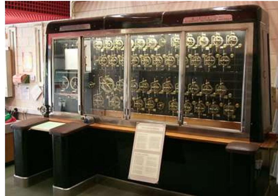
Doodson-Légé Machine (Halved the time of calculations)
